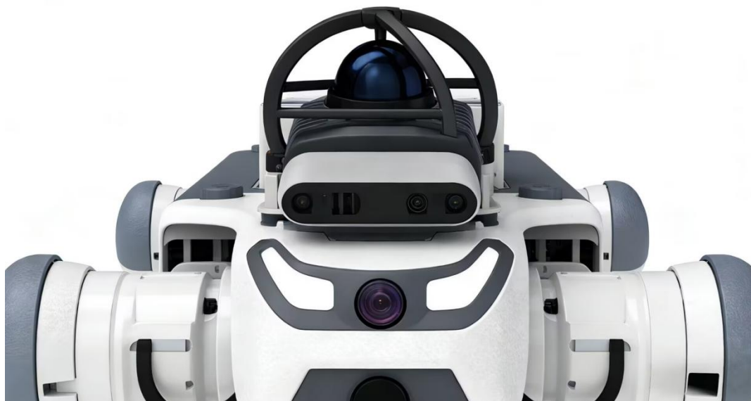
Figure 3: Lidar and camera installation positions
